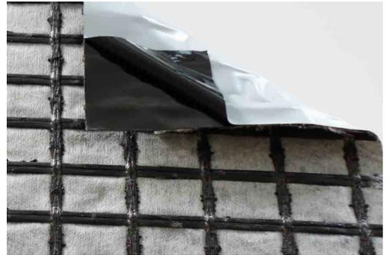
Abb. 1: ADFORS GlasGrid PG/PM Detail Schutzfolie
