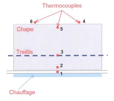
The changes in temperature due to the weather of different thermocouples for each heated test coupon (heat applied below the test coupons) are displayed below.
